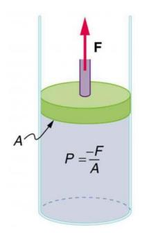
Negative pressure can be reached by pulling on a piston inside a cylinder filled with liquid
